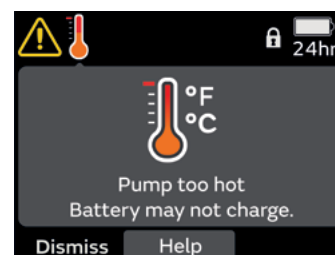
Pump too hot for charging
